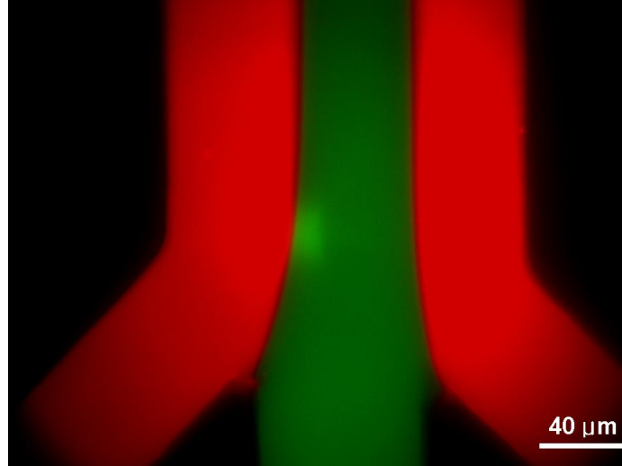
Figure 4.1: Fluorescence image of a microchannel during three-stream flow.
