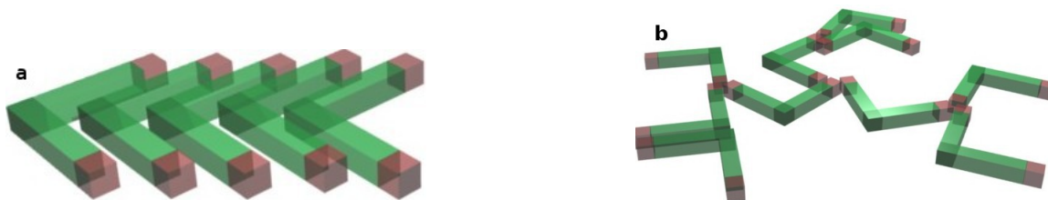
Figure 4.7: Two possible modes of self-assembly for Janus “boomerangs”: (a) geometric, and (b) open and hydrophobic
