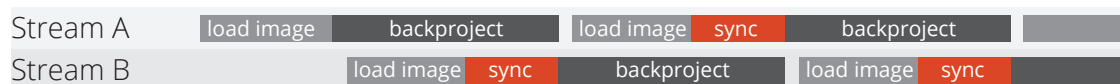
Figure 5.4: Visualisation of the multi-stream approach that hides the latencies for loading the projections on the GPU
