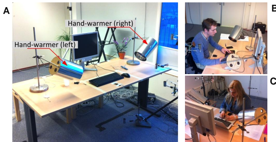
Figure 4.1 (A) Improved local heating system, consisting of two reflector heating lamps, (B) male subject performing office tasks, and (C) female subject performing office tasks.
