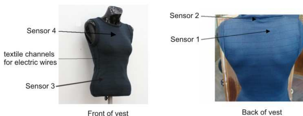
Figure 1. Arrangement of temperature sensors in textronic clothing
