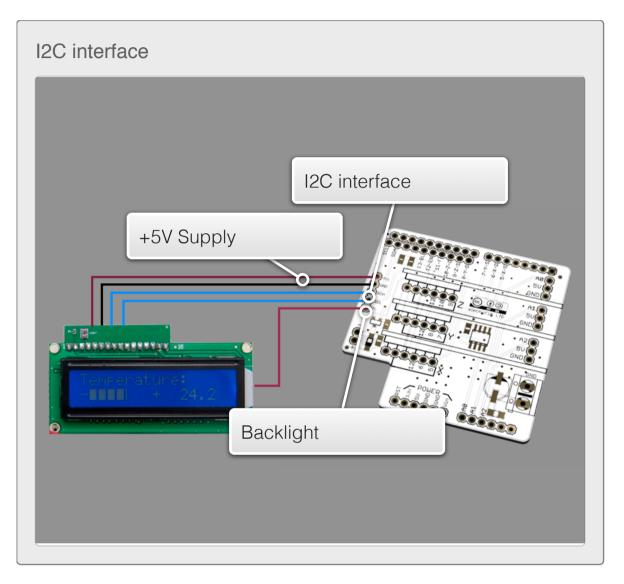
An I2C connector has been added to enable the addition of expansion modules to your CNC controller. The I2C breakout has +5V regulated power supply pins to conveniently power external modules, as well as the I2C's SCL and SDA pins. In addition, this header has IO pin 13 broken out, marked as 13 - BL on the board's silk screen edge (this pin can be used to control a LCD backlight, for example).
