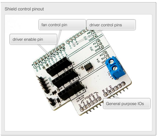
Minimal wiring diagram for the shield is by connecting the stepper drivers, supply and a vinciDuino, Arduino UNO or Leonardo compatible board. That's all you will need to start controlling your CNC machine.
