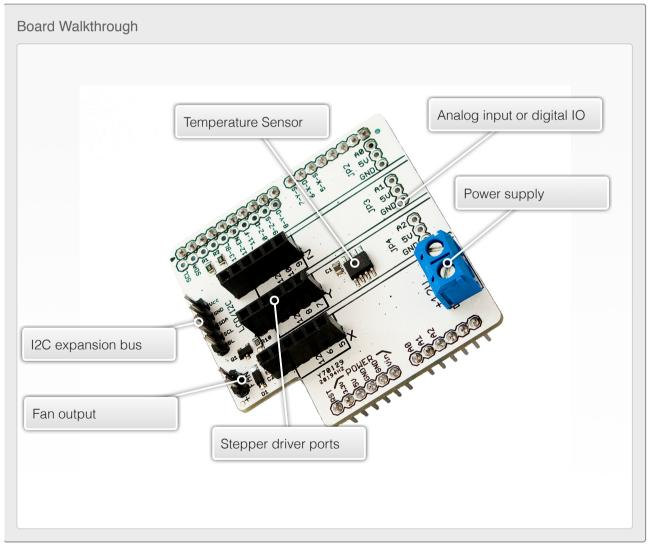
The board has an additional row of pins to make it breadboard friendly.
