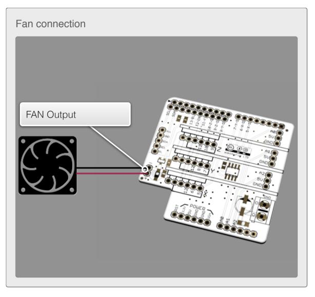
An external fan can be driven using the two pin male header. It is a standard 2.54mm non polarized connector, therefore care must be taken when connecting the fan. Please observe the markings on the PCB.
