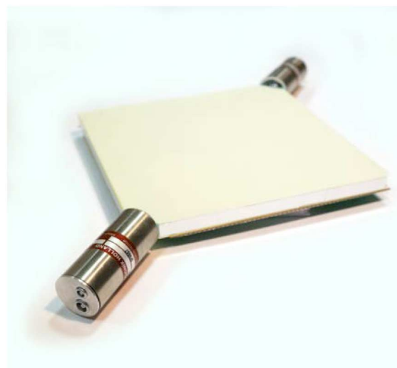
Fig. 2. Assembly of the RTM basic module used in the tests.
