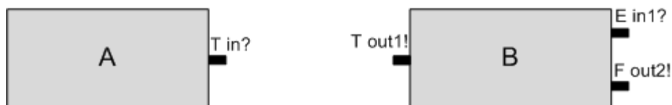
Figure 3 - Components and boundaries. Component A has single right boundary ( in? ) which is an 'inward' boundary of type T. Component B has three boundaries. Its left boundary out1! is an 'outward' boundary also of type T. A's in? and B's out1! boundaries are compatible and may be wired together.
