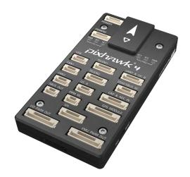
Pixhawk® 4 is the latest update to the successful family of Pixhawk flight controllers. It was designed and developed in collaboration with Holybro and the PX4 team, optimized to run the full Dronecode stack, and comes pre-installed with the latest PX4 firmware.
