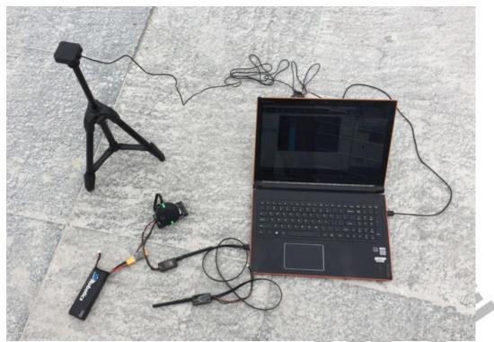
During operation, please place the base station in an outdoor environment with sufficient sky coverage to obtain a good satellite signal. Place the base station on a stable and elevated platform, such as a tripod.
