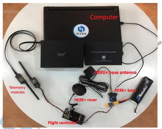
Before using, make sure the hardware is connected correctly:
