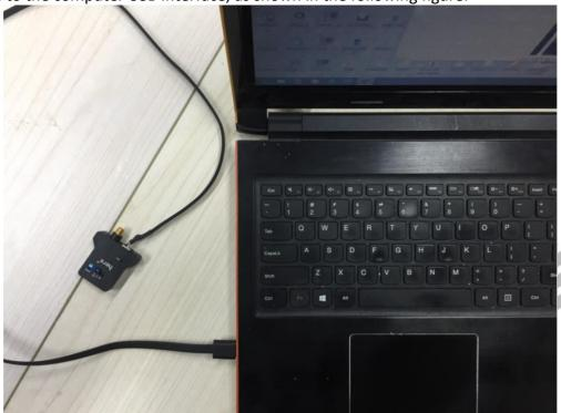
When upgrading a Rover module, use a hexagonal screwdriver to open the case. The rover module has a USB interface connector identical to the base module, you can use the base module USB cable to connect rover to computer. In addition, during the firmware upgrading process, the rover module needs to be powered by connecting to flight controller, as shown in the following figure:
