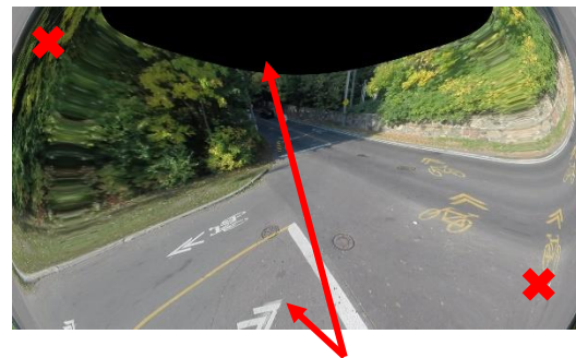
Image clearly not centered: wrong camera resolution set in camera settings
