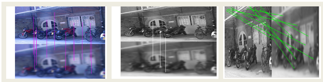
FIGURE 6: Blur comparison. Using group E and F of figure 1. From left to right, the results are: SIFT (10 correct / 10), SURF (3 correct / 3), PCA-SIFT (1 correct / 10), which blur radius is 9.
