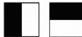
Figure 1. Haar wavelet filters to compute the responses in the horizontal (left) and vertical direction (right). The dark parts have the weight -1 and the light parts +1.
