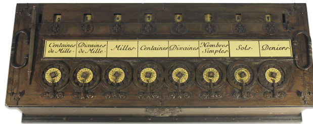
Figure 11: A Pascaline calculator adds numbers using dials, toothed wheels, and falling weights. While incredibly clever, the complicated internal carry mechanism made it unreliable.
