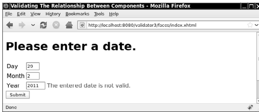
Figure 7–12 Validating a relationship involving three components
