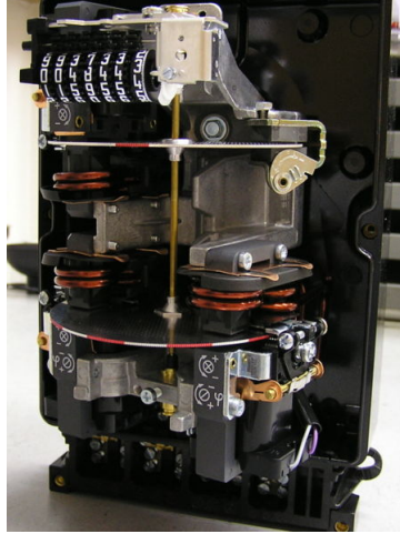
Figure 7: Three-phase electromechanical induction meter (opened) 12
