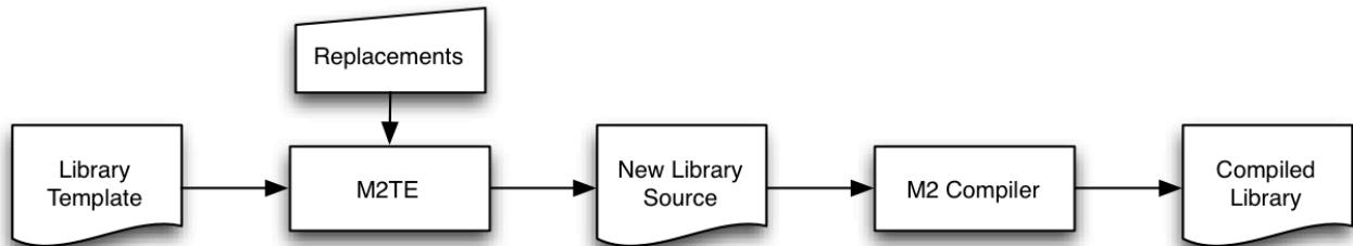
Unlike built-in generics commonly used in other languages, the M2TE utility does not verify whether its input files conform to the syntax of the source language. Doing so would be unnecessary duplication because the generated output will be verified anyhow by a compiler when it is later compiled.
