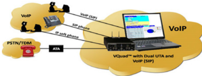
Automated Testing of VoIP (SIP) Interface, Digital VoIP Phones, VoIP Soft-phones using Dual UTA
