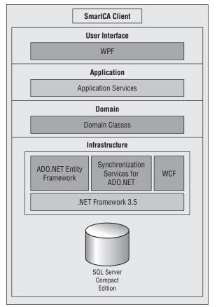
Figure 1.4: The SmartCA application architecture.
