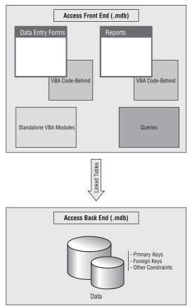
Figure 1.2: Legacy Construction Administration application architecture.
