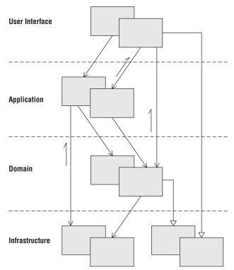
Figure 1.3: The layered architecture (adapted from Evans, 68).
