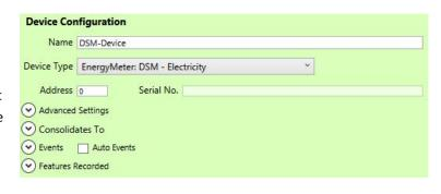
The DSM electricity meter provides separate readings of grid import and export. These readings can be combined with Inverter Yield to produce a total consumption value. Refer to section 6 for details of how to consolidate grid import / export values for use at PVOutput. This section uses DSM grid readings as the basis for the example.
