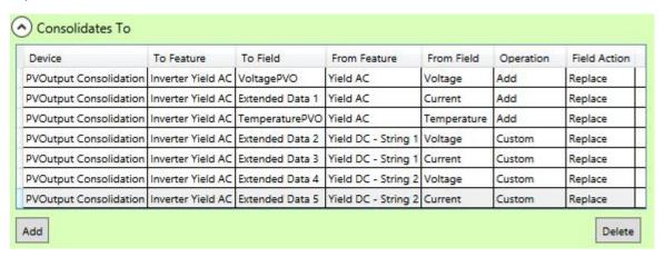
The Consolidates To expander shown above demonstrates how an inverter with two attached strings of panels can consolidate the inverter yield power and energy readings to a PVOutput Consolidation device; and send all AC and DC current and voltage readings to PVOutput.
