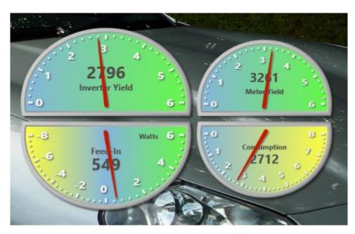
PVMonitor is a Power Monitoring program that comes with PV Bean Counter. It provides four standard gauges and has the ability to display others if required. PVMonitor can be installed on any computer (not just the computer running the main PVBC installation. It communicates with the main PVBC installation using TCP/IP messages.
